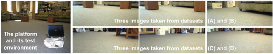
Fig. 2. The Create platform, netbook, and environment in which we tested PixelLaser’s pipeline (left). At right are cropped images from the various test datasets.
